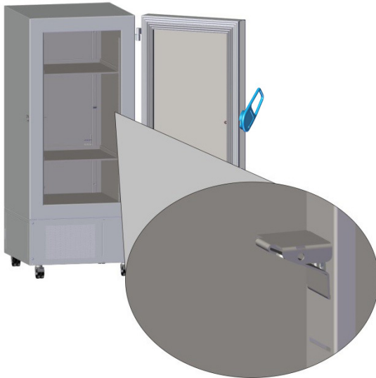
Figure 17: Inserting the shelf holders
