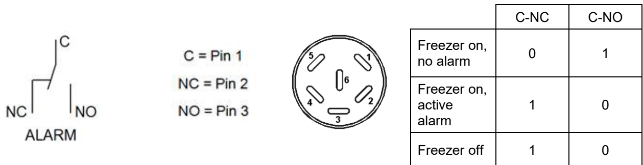
Figure 20: Zero-voltage contacts circuit diagram and pin allocation of DIN socket
