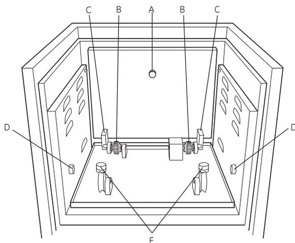
**Fig 2. Hybridization oven drive components**
