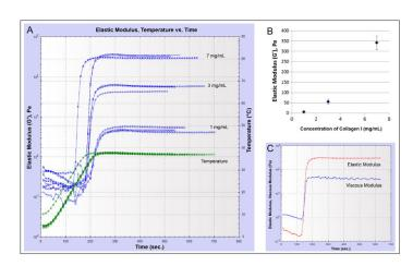
Figure 3. Increase of elastic modulus as a function of Collagen HC rat tail concentration. (A) A plot of the elastic modulus (G') over time for samples of Collagen I at different concentrations. Temperature was ramped from 5°C to 37°C and held at 37°C. (B) Plateau values of the shear modulus (elastic component, G') (Pa) vs. Collagen I concentration (n = 3). (C) Representative time course of elastic modulus and viscous modulus for Collagen I at a concentration of 7mg/mL.
