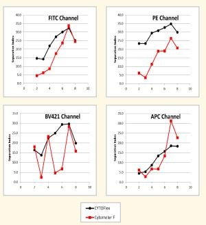
**Figure 5.** Spherotech 8 peak rainbow bead data calculated for a Separation Index between bead peaks as compared to a standard high complexity research cytometer. *Data provided by University of Pittsburgh Cancer Center*
