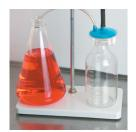
Connect the vacuum tubing to the port marked "VACUUM" on the VacuCap device. Refer to product insert for safety precautions.
