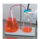
While holding the VacuCap device securely on the filtrate container, start the vacuum. The VacuCap device will seal securely to the container top and fluid will be drawn.
