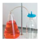
1. Connect the feed tubing to the port marked "INLET" on the VacuCap device. Place the opposite end of the tubing in the unfiltered fluid to be drawn.
