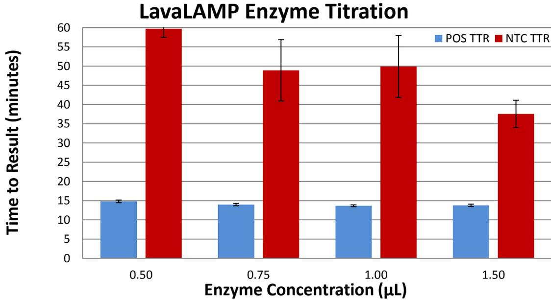
**Figure 3: Enzyme titration using real-time fluorescent detection of amplified products.** Four enzyme concentrations were titrated. Real-time detection was performed on a CFX96 Thermal Cycler (Bio-Rad) in conjunction with Green Fluorescent Dye. In this example, 0.5 µL of LavaLAMP DNA Enzyme provided the lowest background amplification without negatively affecting the positive Time to Result.
