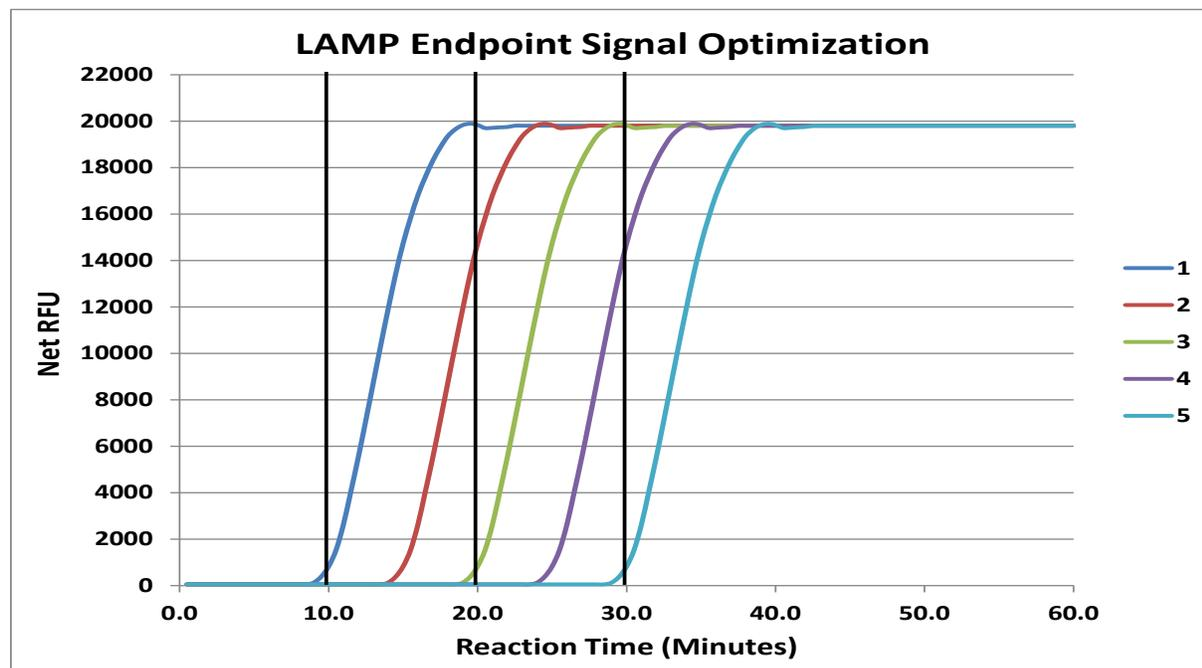
**Figure 10. LAMP Optimization by Endpoint Analysis.** Theoretical product levels from 5 different LAMP Reactions are shown. Measuring the LAMP product (Net RFU) at the suggested endpoints (vertical black lines) allows detection of positive results. With optimization of the LAMP conditions, the LAMP product will reach maximum levels at earlier endpoint time points
