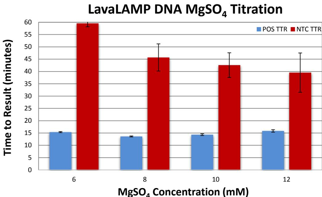
**Figure 2: Magnesium sulfate titration using real-time fluorescent detection of amplified products.** Four  $\text{MgSO}_4$  concentrations were titrated with reactions at 1X, default conditions. Real-time detection was performed on a CFX96 Thermal Cycler (Bio-Rad) with Green Fluorescent Dye. In this example, 6 mM  $\text{MgSO}_4$  provided the lowest background amplification without negatively affecting the positive sample Time to Result.
