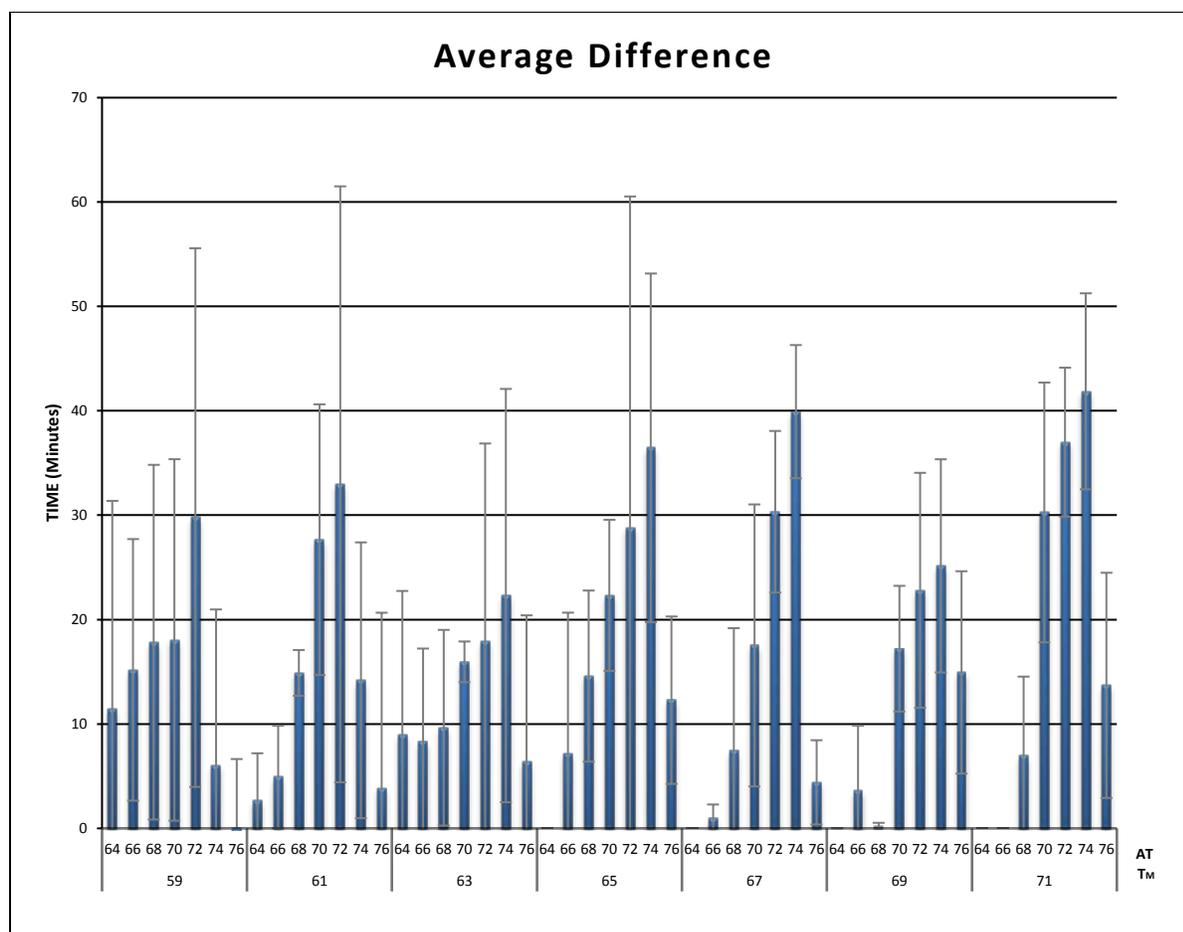
**Figure 9: Effect of Tm setpoints in primer design software.** The difference between the Time to Result of negative and positive samples for various assay temperature (AT) for individual reactions and primer Tm setpoints ("Tm") for FIP and BIP. In this example, the 71°C setpoint provided the largest difference between positive and negative and the largest assay temperature operating window (70°C - 74°C).
