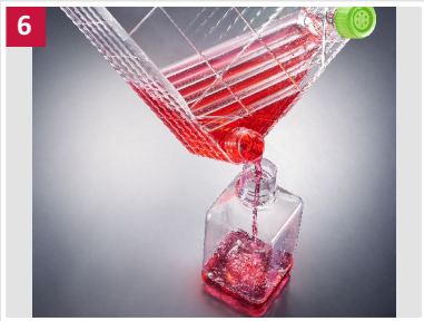
6 Loosen the cap and empty directly into the reservoir
