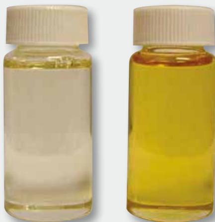
Fig. 2 - Super Refining process (left) removes color and oxidative impurities
