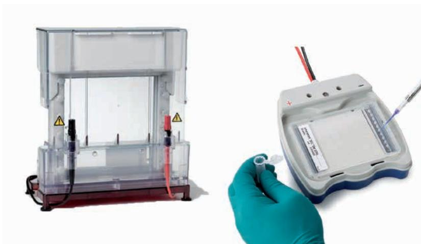
**Fig 3.4.** PAGE is run using either vertical or horizontal formats. SE 400 Vertical Unit (left) and Amersham ECL Gel system (right) are shown as examples. Both systems, and others, are available from GE Healthcare.
