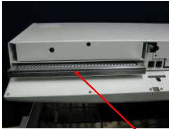
Charcoal Filer behind the bezel
