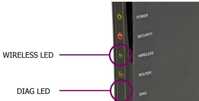
**Figure 20 Wireless router LEDs indicate ready for use**
