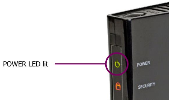
**Figure 19 POWER LED on the wireless router**
