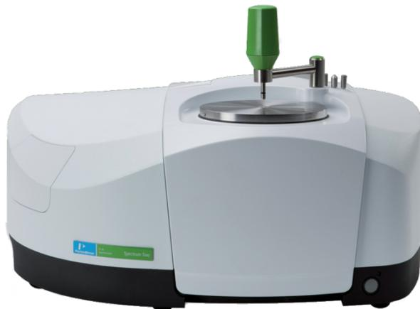
**Figure 8 Spectrum Two FT-IR with Universal ATR Accessory**
