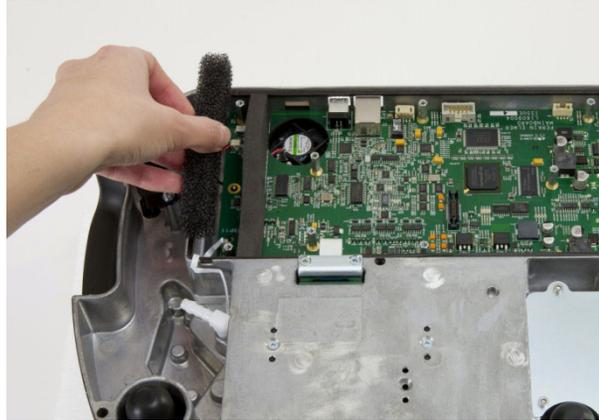
**Figure 94 Remove the used filter**
