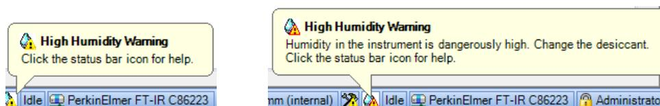
**Figure 72 Humidity sensor High and Critical warning messages**
