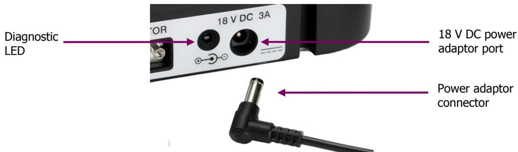
**Figure 18 Power adaptor port on rear of spectrometer**
