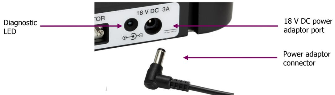
**Figure 12 Power adaptor port on rear of the instrument**
