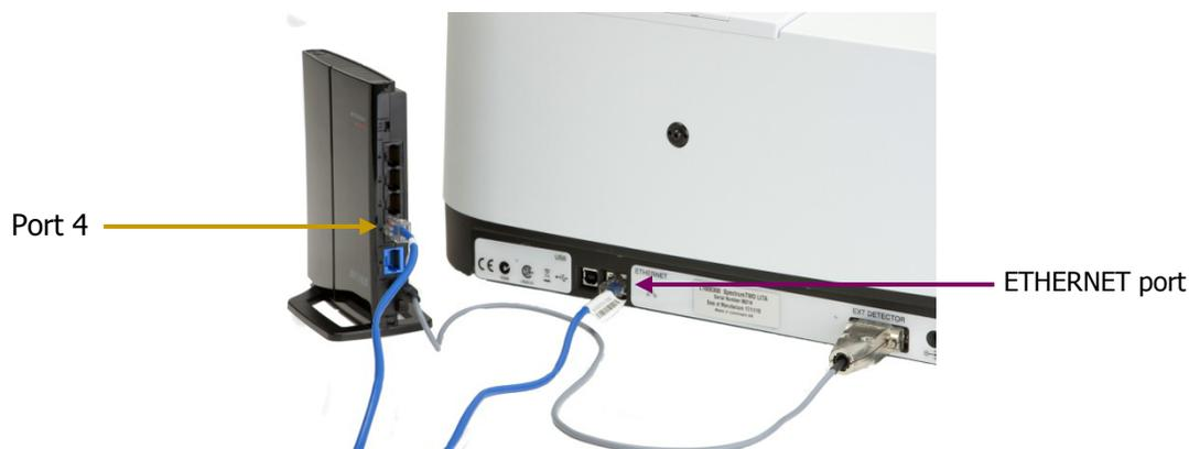
**Figure 17 Ethernet cable connected to Port 4 on the wireless router and the Spectrum Two**
