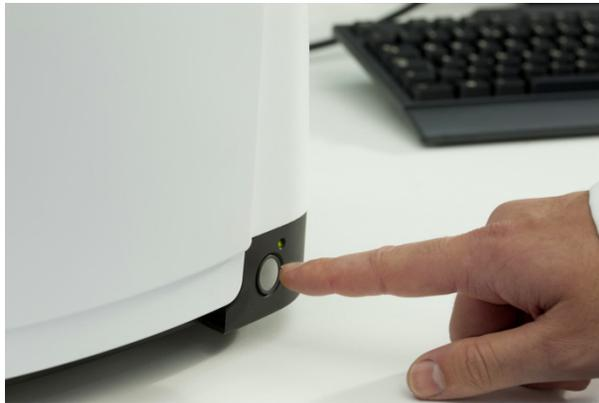
**Figure 73 Power button on the instrument**
