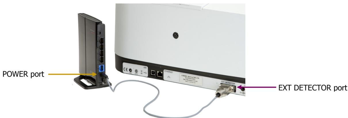
**Figure 16 Wireless router connected to the EXT DETECTOR port**
