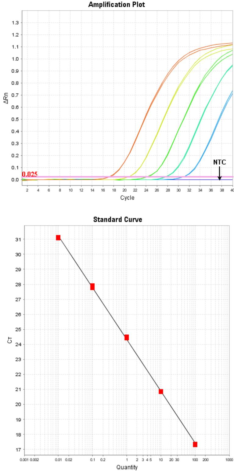
**Figure 1** *Top panel:* StepOnePlus instrument amplification plot using a TaqMan<sup>®</sup> probe. A serial dilution of RNA template (ranging from 0.01–100 ng) was added to each reaction (set up in duplicate) . The fluorescence value used to determine Ct (the threshold line) is shown as a solid line. *Bottom panel:* Standard curve generated from amplification plot. An amplification efficiency of 93.2% and an R-squared value of 0.999 were obtained.
