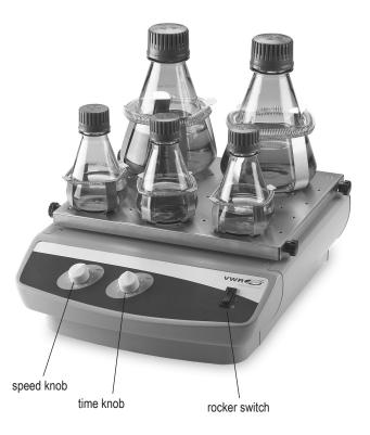
The Standard Orbital Shaker is used for general laboratory shaking needs.
