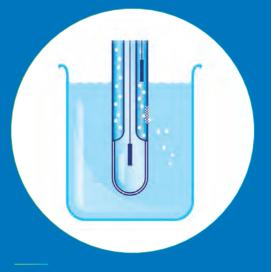
FIGURE 1: Reference and measuring sensor combined in a 2-in-1 sensor.
