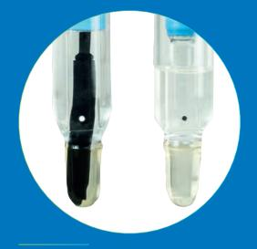
FIGURE 2: Left to right: clean junction (white "dot") in front of a black temperature pro
