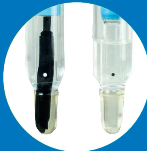
**FIGURE 2:** Left to right: clean junction (white "dot") in front of a black temperature probe
