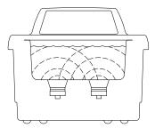
As the sound waves from the transducer radiate through the solution in the tank, they cause alternating high and low pressures in the solution.
