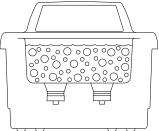
During the low pressure stage, millions of microscopic bubbles form and grow. This process is called CAVITATION, meaning "formation of cavities".
