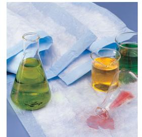
Deluxe pads are more absorbent and thicker with more absorbent cellulose fluff than standard pads. Super deluxe pads have an added polymer that absorbs more moisture. Super deluxe pad 56617-032 comes in a breathable format.
