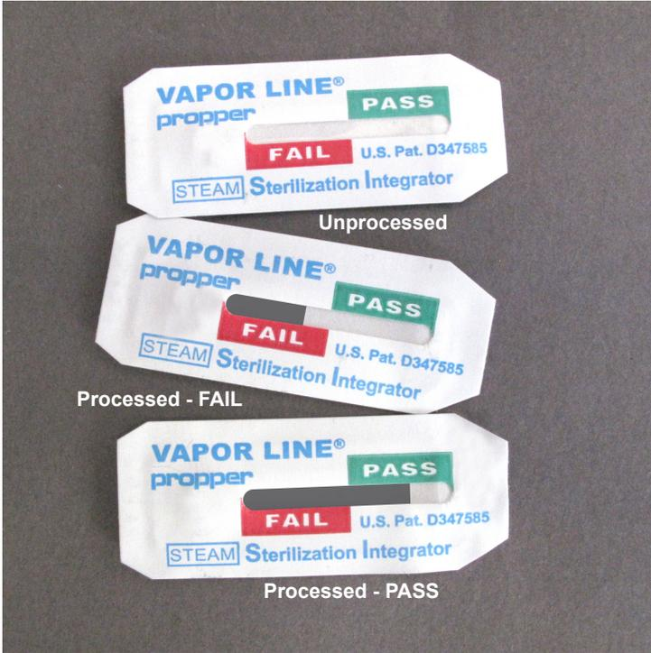
The Vapor Line® integrator is a chemical indicator for monitoring the essential conditions of steam sterilization processes - saturated steam, temperature, and time in gravity displacement and pre-vacuum sterilizers operating in the 250°F - 272°F temperature range.
