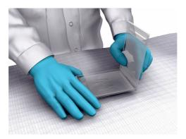
Hold the gel cassette bottom plate over a container with suitable buffer, with the gel facing downwards. Gently push a tweezer between the gel and the cassette bottom plate until the gel is removed from the bottom plate.
