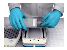
Remove the top plate from the gel cassette and allow the gel to sit on the bottom plate.
