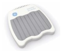
The safety lid has two magnets which will activate current only when their magnetic fields are in contact with the electrodes inside the base unit of Amersham ECL Gel Box. This means that Amersham ECL Gel Box is only powered when the safety lid is in the correct position. Removing the safety lid will switch off the high voltage to the electrodes.
