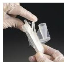
Clip top of funnel and base together.
