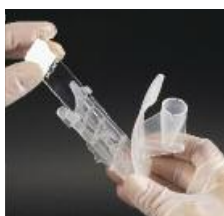
Insert microscope slide.
