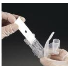
Place new filter onto microscope slide.
