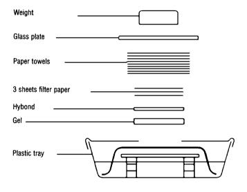
Figure 1. Diagrammatic representation of a capillary blotting apparatus
