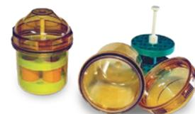
To help minimize contamination from broken or leaking tubes. Clear plastic allows for viewing from top to bottom. Each canister seals with an O-ring and is autoclavable up to 121°C.
