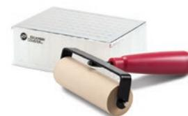
Use roller (VWR Cat. No. BK538618) to ensure complete plate sealing.
