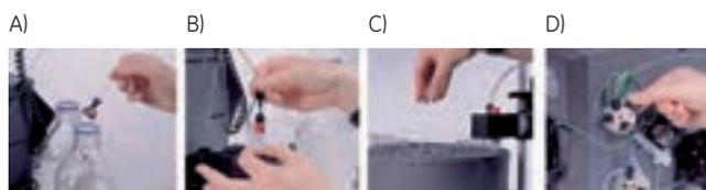
Fig 2.8. Typical procedures using ÄKTApurifier plus. (A) Prepare the buffers. (B) Connect the column. (C) Prepare the fraction collector. (D) Load the sample and press start.
