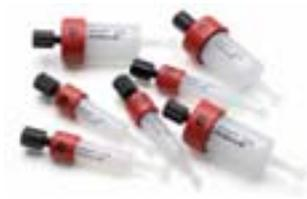
Fig 7.21. HiTrap prepacked columns.
