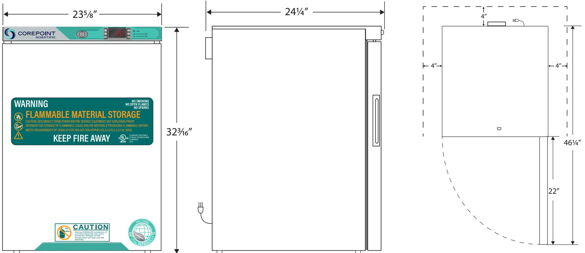
**NOTE: Ventilation Requirements – Minimum 4" clearance on sides and back**
