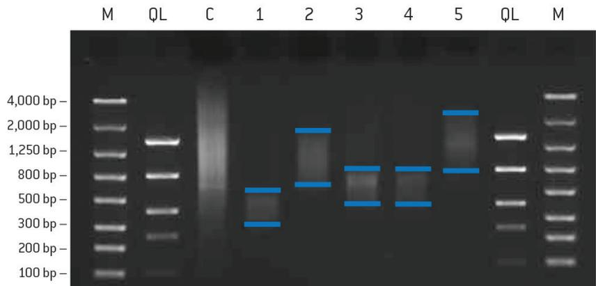
**Figure 2: Recovered samples of various size selections**
