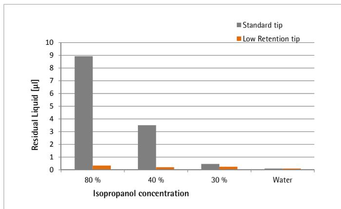
**Figure 2. Effect of liquid surface tension to the amount of residue in the tip.** 1000µL of various concentrations of isopropanol (30%, 40%, 80%) and distilled water were aspirated and dispensed with both Sartorius standard and Low Retention Optifit Tips (1000µL) using Sartorius Picus® electronic pipette (1000µL). The residual liquid in the tips was measured using the gravimetric analysis method described in the Materials and methods. The test was repeated for 10 tips of each manufacturer.
