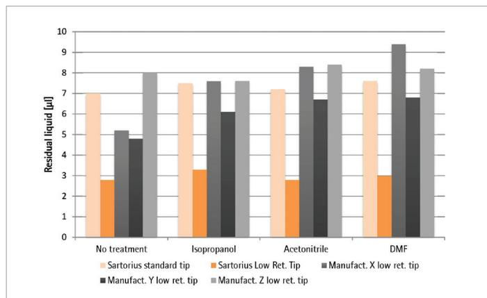
**Figure 3. Comparing the chemical resistance of low retention pipette tips** Low retention tips from three manufacturers were compared with Sartorius standard and Low Retention Tips. The test for chemical resistance was performed as described in the Materials and methods using 1000µL pipette tips with Sartorius Picus® electronic pipette (1000µL). The test was repeated for six tips of each manufacturer.
