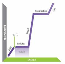
Specific Latent heat capacity varies depending on the specific elements and phase change (ie.melting, vaporization, fusion) involved. At 37°C, over a 1°C temperature range and due to the latent heat caused by transitioning between a liquid and a solid phase, PCM's actually hold over 40 times the energy, by volume, than water:
