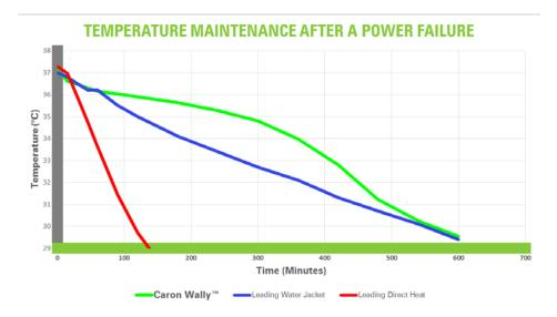
When running at 37°C and presented with a power failure, the Wally CO<sub>2</sub> incubator maintains temperature above 30°C slightly longer (roughly 9 hours) than even the industry-
