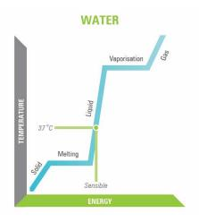
Specific heat capacity depends on material density, with denser materials (such as water) offering greater Sensible capacity than less dense substances (such as air).
