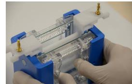
4) Insert into casting base. Push the cams into the holes in the insert. Turn cams about 90° or until tight. Do not over tighten.
