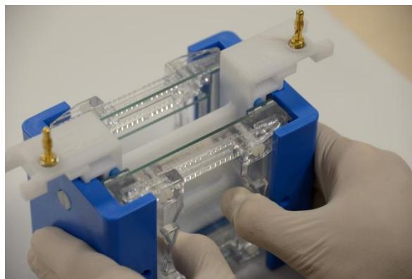
4. Position the PAGE Gel Insert on a flat surface. **Do not insert the PAGE gel Insert into the casting base at this point.**
