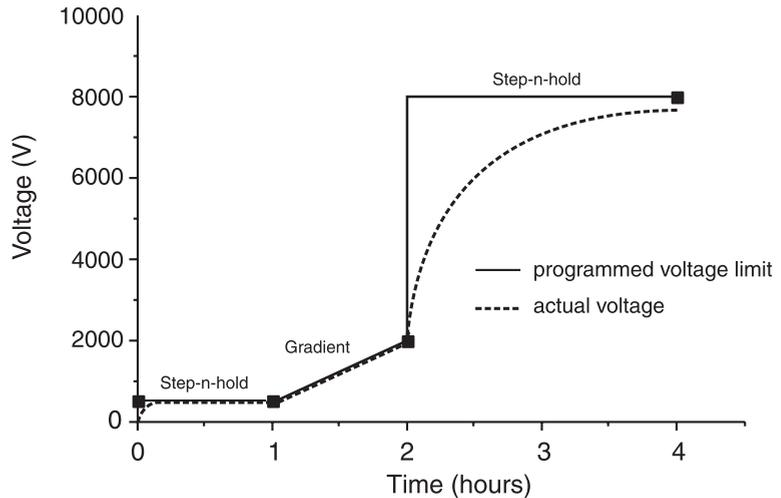
**Note:** *The set voltage is the voltage limit. Under conditions of limiting current, it may take some time for the maximum voltage to be reached, and under certain power conditions, it may not be reached at all.*
