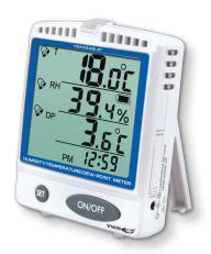
**Traceable to NIST**—To assure accuracy an individually serial-numbered Traceable Certificate is provided from an ISO/ IEC 17025:2005 (1750.01) calibration laboratory accredited by A2LA. It indicates traceability to standards provided by NIST (National Institute of Standards and Technology).
