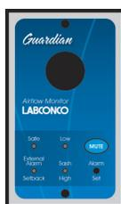
**Guardian™ Airflow Monitors.** Sense and alert you to low airflow conditions. From the monitor's face plate, you can easily select and calibrate a set point between 30 and 250 fpm using a velocity meter and a screwdriver. Audible/visual alarm. Include night setback, external alarm and alarm mute functions. Flush-mount design. **Requires field calibration.**
