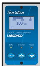
**Guardian™ Digital Airflow Monitors.** Sense and alert you to low airflow conditions. LCD displays actual airflow in fpm or m/sec. Audible/visual alarm alerts you to sustained low velocity condition. LCD displays calibration instructions. Contact Labconco for optional temperature sensor or optional RS-485 port for Modbus\*\* RTU communication. Flush-mount design. **Requires field calibration.**
