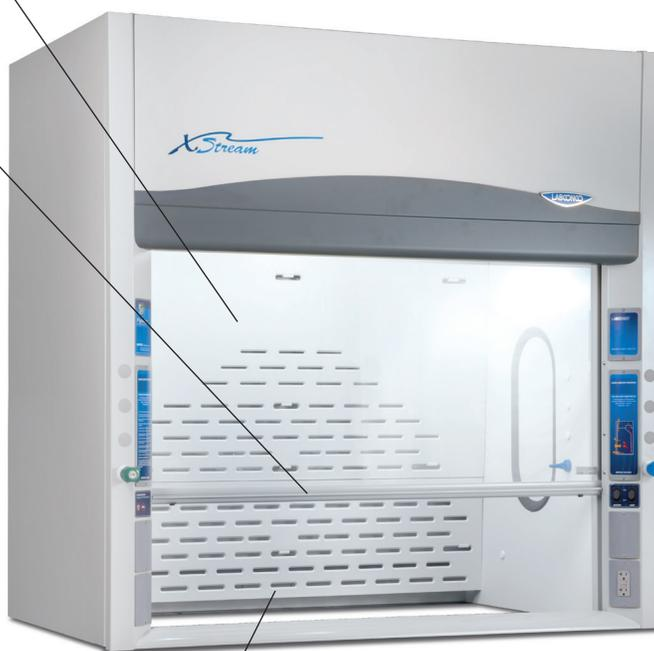
❖ **Eco-Foil™ air foil\*** reduces energy consumption by 7-10% compared to flat air foils. Aerodynamic curve allows air to sweep the work surface maximizing containment. Clean-Sweep™ openings pull inflow air from under the air foil forcing air into non-turbulent air streams. Curve is comfortable for resting arms.
